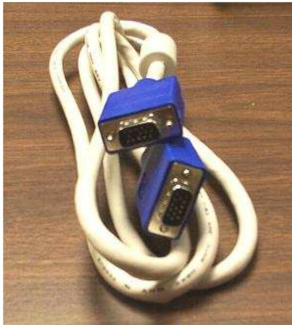
5. Plug one end of the VGA cable into the 15 pin "monitor out" jack of the laptop. It is the blue colored jack on the right side of the computer shown in the picture below.
