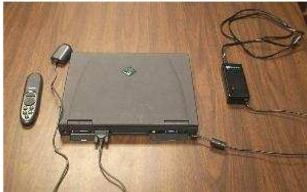
2. The above picture shows a typical setup for a laptop computer. The black box and cable to the right of the computer is the power supply. Connect the power supply to the 9-12 VDC jack. See picture below to see what jacks to plug into.
